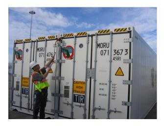
Inserting head of GM121 End Lock Wand into correct inside edge hole of corner casting.
