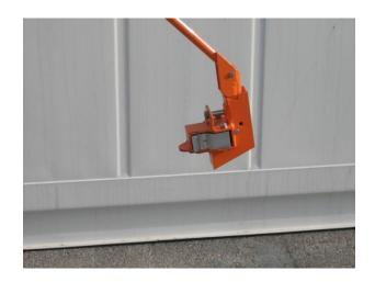
Head and jaw of the GM184 Top Access End Lock Wand
