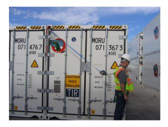
GM121 End Lock Container Wand locked into corner casting and worker positioned correctly one container wide away.
