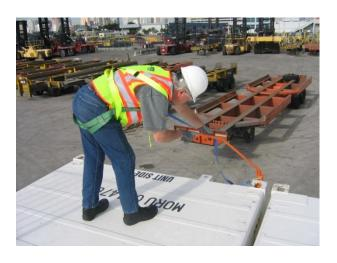
Inserting GM184 Top Lock Access End Lock Wand into end hole of corner casting while standing 3' from the end side leading edge.
