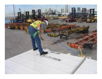
Worker working correctly one container width away and unlocking twist locks below with telescopic pole.
