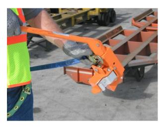
Connecting a couble lock snap of SRL to anchor point of GM184 Top Access End Lock Wand.
