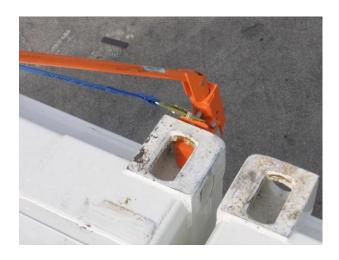
GM184 Top Access End Lock Wand locked into end hole of corner casting.
