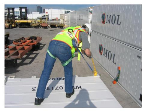
Inserting GM120 Top Lock Wand into corner casting while standing 3' from the end and side leading edge.
