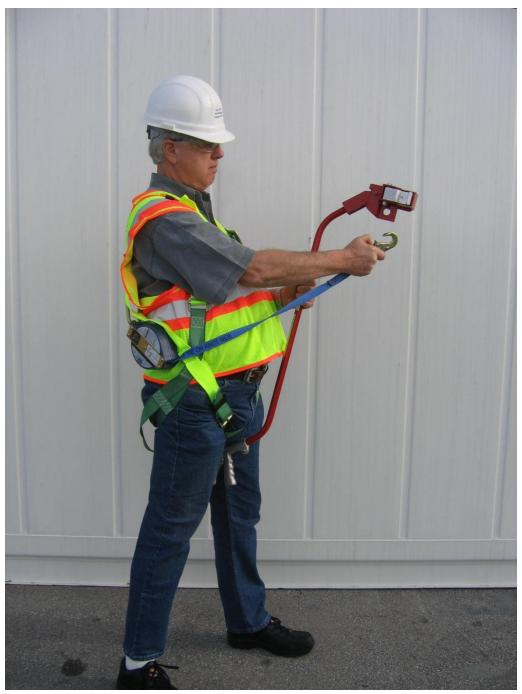
Connecting double lock snap of SRL to anchor portion of GM121 End Lock Wand.
